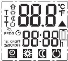
To start the controller fit two “AA” batteries in the battery compartment. Once batteries are fitted all symbols will be displayed on the LCD screen as shown.
